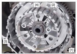
Apply engine oil to a new clutch center lock nut threads and seating surface.
