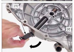
Install the right crankcase cover [1] by holding the clutch lifter lever [2].
