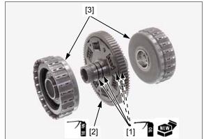
Apply engine oil to the needle bearings in the primary driven gear.
