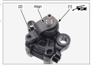
Install the adjuster lock nut [1].
