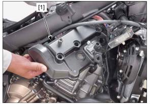
Install the bolts [1] and tighten them to the specified torque.
