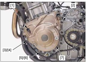
Remove the dowel pins [1] and oil joint [2].
