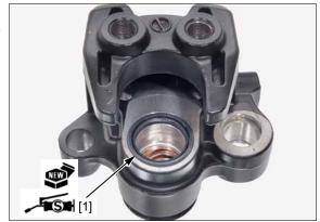
Apply 0.4 g minimum of silicone grease to the parking brake shaft outer surface.
