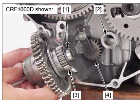
Line up the rear balancer driven gear and sub gear teeth by inserting a suitable pin [1] into the holes of gears.
