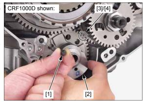
Install the dowel pins [1].
