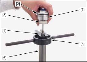
Pour out the fork fluid by pumping the outer pipe [1] several times.
