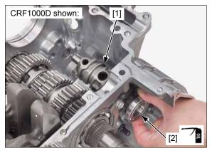
Apply locking agent to the shift drum bearing setting bolt threads (page 1-20).
