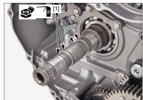
Install the dual clutch assembly [1] onto the mainshaft, being careful not to damage the seal rings.
