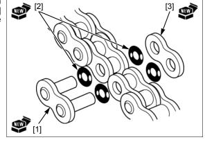
Make sure that the master link pins [1] are installed properly.
