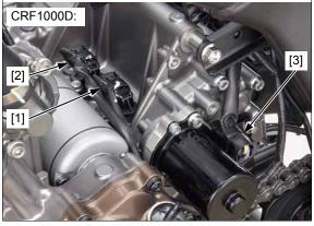
Install the bracket [1] and bolts [2], and tighten the bolts securely.
