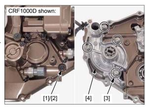
Install a new O-ring [1] into the groove in the water pump body [2].
