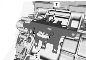
Install the O2 sensor wire clip [1] to the connector clip stay.
