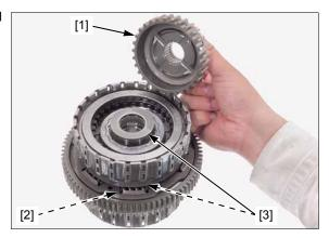
Remove the clutch assemblies [1] and O-rings [2] from the primary driven gear.
