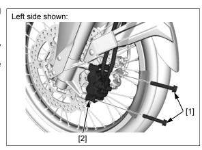
ED model: Remove the axle cap [1].
