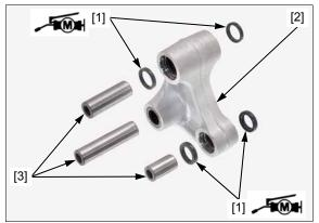
Install the collar [1] into the cushion connecting rod [2].
