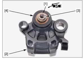
Apply 0.4 g minimum of silicone grease to the push rod rolling surface and piston sliding surface.
