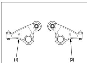
Apply molybdenum oil solution to the rocker arm sliding area and thrust surface.
