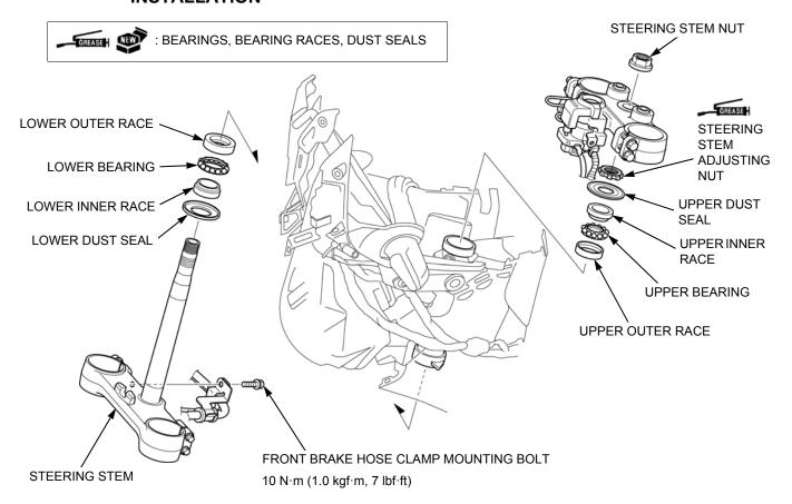
Apply specified grease (page 1-23) to the upper and lower bearings and bearing races.
