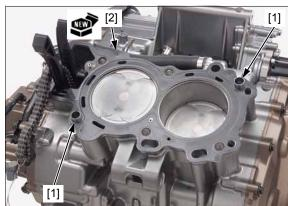
Route the cam chain [1] through the cylinder head and install the cylinder head [2] onto the cylinder.
