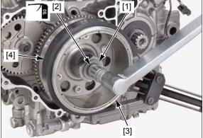
Apply molybdenum oil solution to the starter reduction gear shafts outer surfaces.
