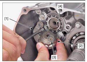
Apply locking agent to the threads of the shift drum center bolt [1] (page 1-21).
