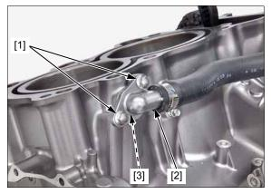
CRF1000D: Remove the cam chain tensioner pivot bolt [1], cam chain tensioner [2], and washer [3].
