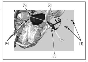
Always turn the ignition switch OFF before removing the battery.
