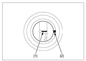
Install the valve lifters [1] and shims [2].
