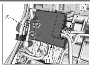
Install the alternator assembly wire onto the frame:
