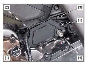
Remove the bolt [1] and set plate [2].
