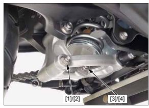
Remove the shock absorber upper mounting bolt [1] and nut [2].
