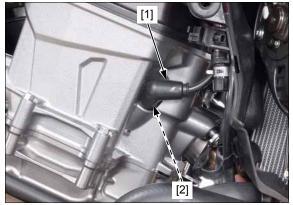
Remove the spark plug cap [1].
