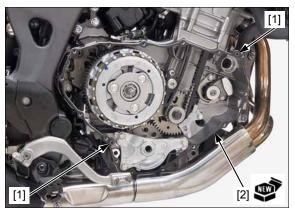
Coat a new O-ring [1] with engine oil and install it onto the groove of the water pump cover.
