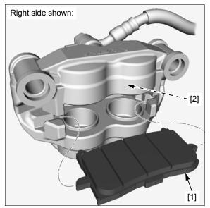
Install the brake caliper [1] and new mounting bolts [2]. Tighten the bolts to the specified torque.
