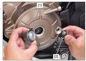
Rotate the crankshaft counterclockwise and align the "T1" mark [1] on the flywheel with the index mark [2] on the alternator cover.
