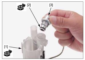
Install a new O-ring [1] to the fuel pump [2]. Install the fuel pump.
