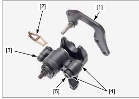
Remove the adjuster lock nut [1] while holding the brake arm [2].
