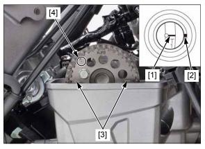
Remove the rocker arm shaft stopper bolt [1], sealing washer [2], and rocker arm shaft bolts [3].
