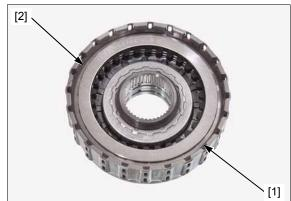
Coat new O-rings [1] with engine oil and install them into the grooves in the primary driven gear [2].
