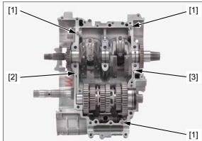
Apply molybdenum oil solution to the main journal bearing sliding surfaces on the lower crankcase. Install the lower crankcase onto the upper crankcase. Make sure the upper and lower crankcases are seated securely.
