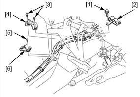
CRF1000D: Remove the bolt [1] and parking brake cable guide [2].
