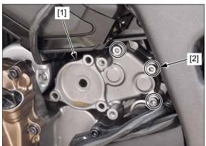
Coat a new O-ring [1] with engine oil and install it into the groove in the shift control motor [2].
