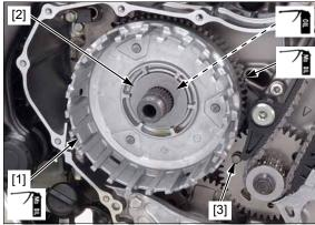
Install the clutch center [1], washer [2], and lock washer [3].
