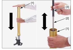
Slowly push the outer pipe [1], and gently seat the dust seal [2] onto the axle holder [3] and leave it for 5 minutes.
