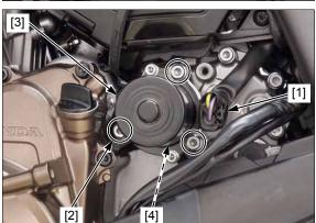
Remove the torx bolts [1] and reduction gear cover [2].
