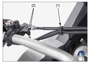
CRF1000D: Install the wire clamp [1] and connect the parking brake switch connectors [2].
