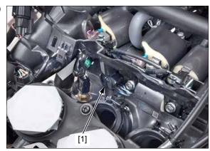
Releasing the bosses [1] from the grommets [2] by pulling the ignition coil tray assembly [3] rearward, and remove the tray assembly.
