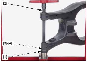
Remove the needle bearing (24 x 31 x 28 mm) [1] out of the right pivot using the special tool.
