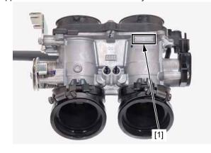
The color label [1] is attached on the up side of the ETC tray. When ordering color-coded parts, always specify the designated color code.
