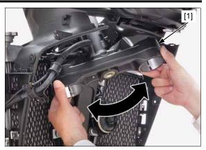
Retighten the steering stem adjusting nut [1] to the specified torque using a special tool.
