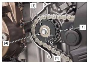
Install the stay [1] and bolt [2], and tighten the bolt securely.
