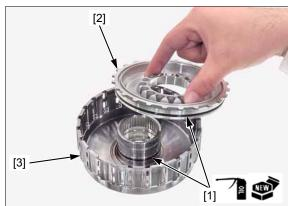
Coat a new O-ring [1] with engine oil and install it into the return spring retainer groove.
