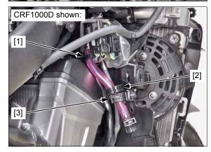
Loosen the connecting hose band screws [1]
