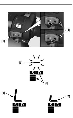
4. Start the engine and let it idle. The "-" [1] on the shift indicator starts blinking an interval of 2 seconds. The Clutch Initialize Learning is successful, when the "-", "D" and "S" indicators [2] go off. Stop the engine.
