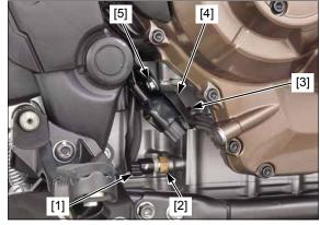
Remove the drive sprocket bolt [1], washer [2], and drive sprocket [3] from the countershaft and drive chain.
