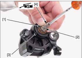
Apply 0.4 g minimum of silicone grease to the brake shaft boot lips.
