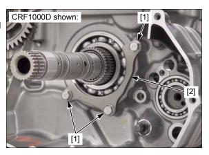
Remove the right mainshaft bearing [1] from the upper crankcase.
