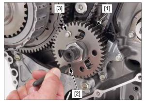
Remove the dual clutch assembly [1] from the mainshaft.
