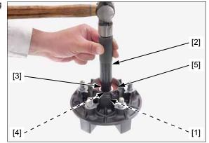
Replace the wheel bearings in pairs. Do not reuse old bearings.
