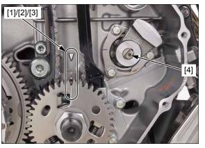
Rotate the water pump shaft and align the shaft slit with the pump cover index line as shown.
