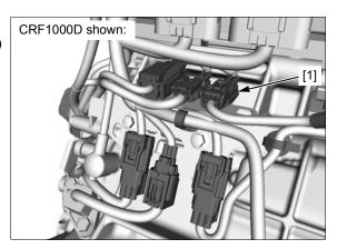
Check for continuity between the rear brake light switch 2P (Gray) connector [1] terminals.
