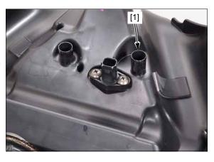
Temporarily install the fuel tank (page 7-6). Temporarily connect the IAT sensor 2P (Black) connector (page 7-12).
