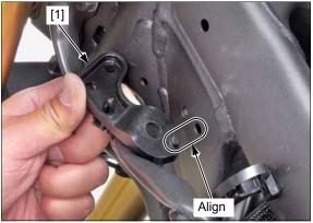
Install the bolt [1] and tighten it securely. Install the wire clips [2] to the stay [3]. Install the wire band [4].
