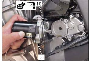
Install the torx bolts [1] and tighten it to the specified torque.
