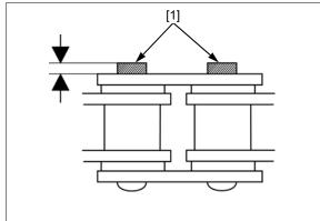
Make sure that the pins are staked properly by measuring the diameter of the staked area using a slide caliper [1].
