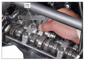
Rotate the crankshaft counterclockwise 270° and align the "T2" mark [1] with the index mark [2].
