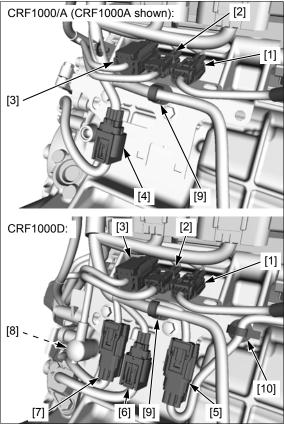
Remove the bolts [1] and connector clip stay [2].
