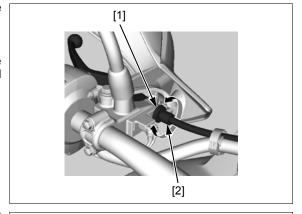
Major adjustment is made with the lower adjusting nut [1] at the clutch lifter arm.
