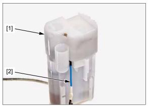
Install a new O-ring [1] to the fuel pump stay [2].
