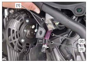
Loosen the hose band screws [1] and disconnect the upper radiator hose [2] and radiator hose B [3] from the left radiator.
