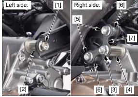
Remove the swingarm pivot nut [1], pivot bolt [2].
