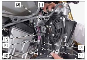
Loosen the hose band screws and disconnect the lower radiator hose [1], radiator hose A [2], and B [3] from the right radiator.
