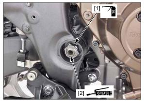
Tighten the rear lower nut (10 mm) [1] to the specified torque.
