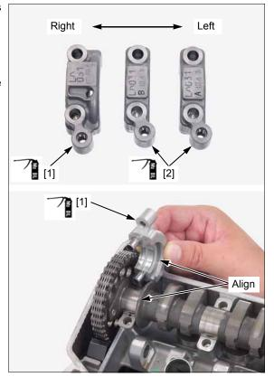
Apply engine oil to the camshaft holder bolt [1] threads and seating surfaces and install them.
