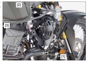
Disconnect right fan motor 2P (Black) connector [1] and remove the right radiator assembly [2].
