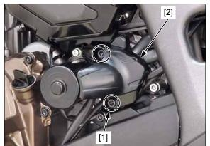
Disconnect the shift control motor 2P (Black) connector [1].
