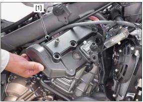
Remove the plug pipe seals [1] and cylinder head cover packing [2].
