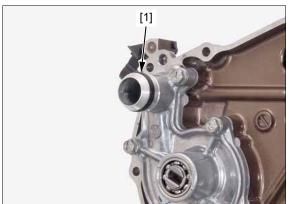
Check the bearings and replace if necessary (page 13-55).
