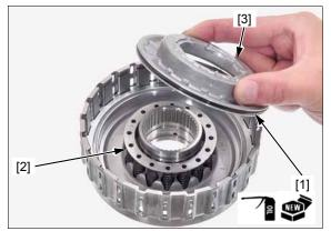
Place the snap ring [1] onto the clutch.
