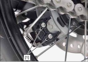
Remove the socket bolts [1] and parking brake caliper cover [2].
