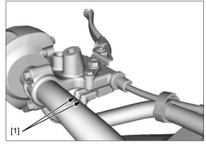
Remove the bolts [1], holder [2], and parking brake lever assembly [3].
