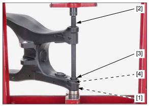
Remove the needle bearing [1] out of the left pivot using a hydraulic press and special tool.
