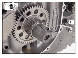
Clean any oil from the crankshaft and flywheel tapered area thoroughly.
