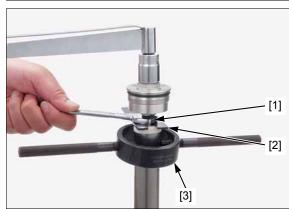
Tighten the fork bolt after installing the fork slider into the steering stem.
