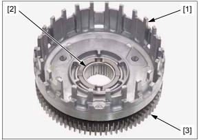
Inspect the following parts for scratch, damage, abnormal wear and deformation. Replace if necessary.
