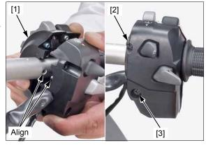
CRF1000/A: Install the clutch lever assembly [1] by aligning its end with the paint mark [2] on the handlebar.
