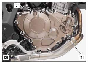
Remove the dowel pins [1] and gasket [2].
