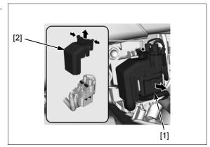
Disconnect the starter relay switch 4P (Black) connector [1].
