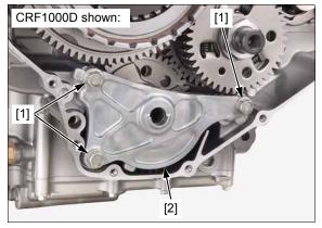
Remove the dowel pins [1].
