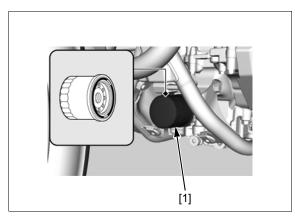
Check the oil filter boss [1] protrusion from the crankcase is within the specified length as shown.
