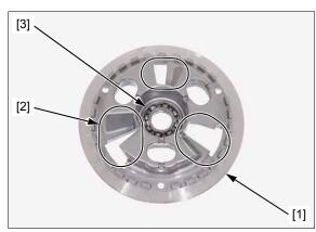
Check the following of the clutch center [1] for scratch, damage, abnormal wear and deformation.
