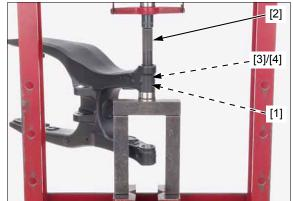
Apply molybdenum disulfide grease to a new needle bearing rotating area.
