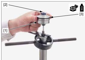
Be careful not to damage the fork bolt when tightening
