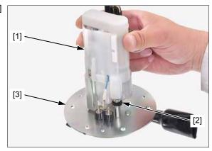
Remove the chamber [1] by releasing the tabs [2].
