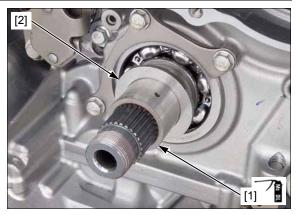
Apply engine oil to the clutch outer needle bearing. Apply molybdenum oil solution to the primary driven gear teeth and clutch outer sliding area.
