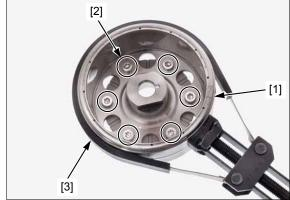
Remove the starter clutch assembly [1].
