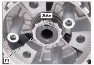
Apply molybdenum oil solution to the entire surface of judder spring seat and judder spring.
