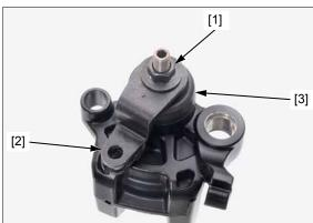
Remove the push rod [1] while holding the brake shaft
