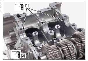
Apply molybdenum oil solution to the thrust surfaces of the crankshaft as shown.
