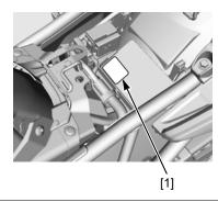
The registered number plate (ED, RU models) [1] is attached on the right side of the rear frame.
