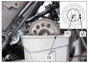
Check the No.2 cylinder intake valve clearances by inserting a feeler gauge [1] between the valve lifter and cam lobe.
