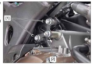
Install the left/right heel guards [1] and bolts [2], and tighten the bolts securely.
