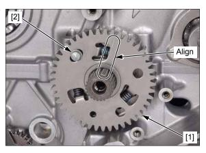
Install the timing sprocket [1] with its punch mark [2] facing out as shown
