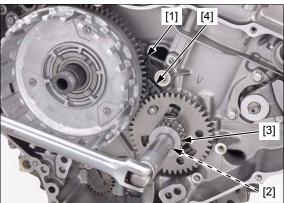
Remove the timing sprocket [1].
