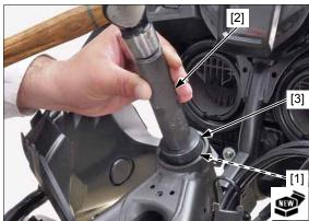
Drive in a new lower outer race [1] using the special tools.
