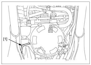
Disconnect the turn signal light relay 18P (Black) connector [1].
