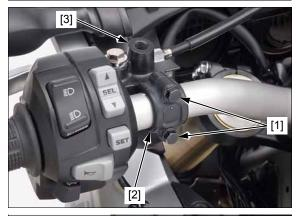
CRF1000D: Remove the bolts [1], holder [2], and parking brake lever assembly [3].
