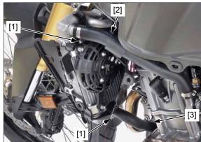
Disconnect left fan motor 2P (Black) connector [1] and remove the left radiator assembly [2].
