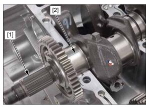
Install the dowel pins [1].
