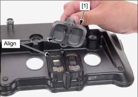
Remove the PAIR reed valves [1] and port plates [2]. Installation is in the reverse order of removal.
