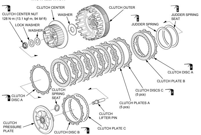
Apply molybdenum oil solution to the clutch outer guide entire surface.
