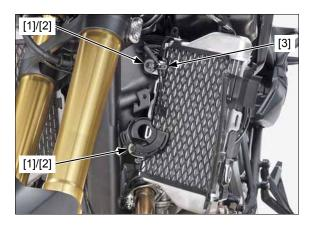
Release the connector clip [1] from the radiator shroud. Release the air cleaner housing drain hose [2] from the clamp [3].
