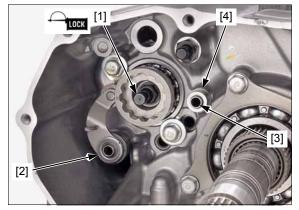
Install the plunger springs [1], plungers [2], and ratchet pawls [3] into the drum shifter [4] and set them in the drum shifter guide plate [5].
