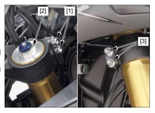
When disassembling the fork, turn the pre-load adjuster [1] and rebound adjuster [2] counterclockwise to the softest position (be sure to record the number of turns from the starting position).
