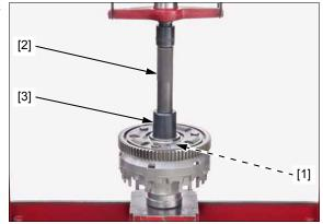
Coat a new needle bearing with engine oil.
