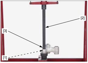
Never install the old bearing, once the bearing has been removed, the bearing must be replaced with a new one. Apply molybdenum disulfide grease to new needle bearings rotating area.
