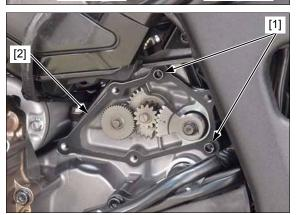
Install the reduction gear cover [1] and torx bolts [2], then tighten the torx bolts.
