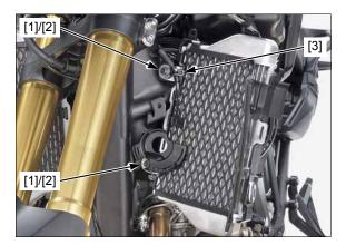
Release the connector clip [1] from the radiator shroud. Release the air cleaner housing drain hose [2] from the clamp [3].
