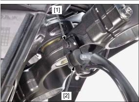
Loosen and remove the steering stem adjusting nut [1] using the special tool.
