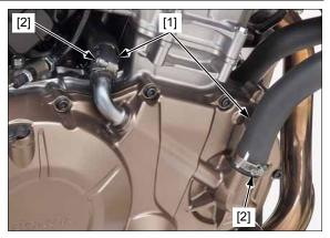
Connect the clutch cable [1] with the clutch lifter lever [2].
