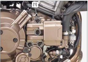
Connect the linear solenoid valve 4P (Black) connector [1].
