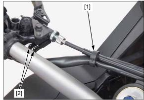
Apply grease to the throttle pipe flange groove.
