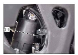
Install the rear brake hose B [1] and rear wheel speed sensor 2P (Black) connector [2] through the hole [3] of rear fender B.
