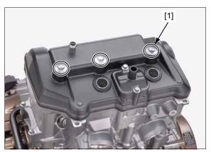
Remove the cylinder head cover [1] to the right side as shown.
