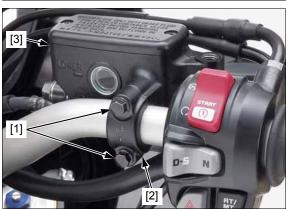
Remove the screw/washers [1] and separate the right handlebar switch housing [2].
