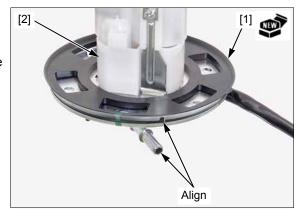
Install the fuel pump unit [1] into the fuel tank.
