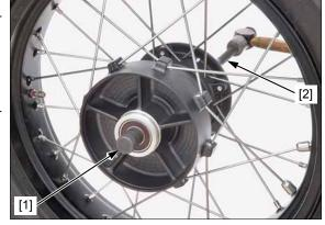
bearing, once the fully seated. bearing has been removed, the bearing must be replaced with new ones.
