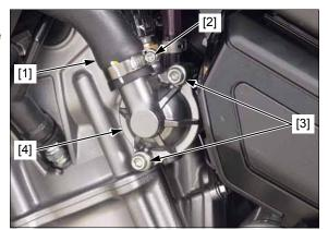
Remove the thermostat [1] from the upper crankcase. Installation is in the reverse order of removal.
