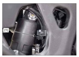
Remove the bolt [1] and release the sensor wire [2] from the brake hose clamp [3].
