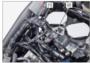
Disconnect the throttle body by pulling it upward.
