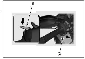
4. The self-diagnostic memory is erased if the shift indicator "-" goes off and starts blinking as shown.
