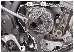
Remove the lock washer [1], washer [2], and clutch center [3].
