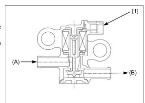
Measure the resistance at the 2P connector [1] of the PAIR control solenoid valve.
