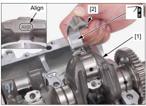
Apply engine oil to new crankpin bearing cap bolt threads and seating surfaces.
