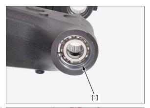
Remove the ball bearing 6003 [1] out of the right pivot using a hydraulic press and special tool.
