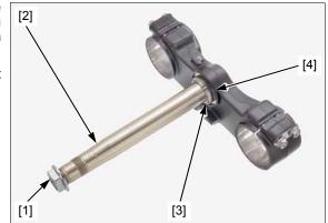
Apply specified grease to a new lower dust seal lips (page 1-23).
