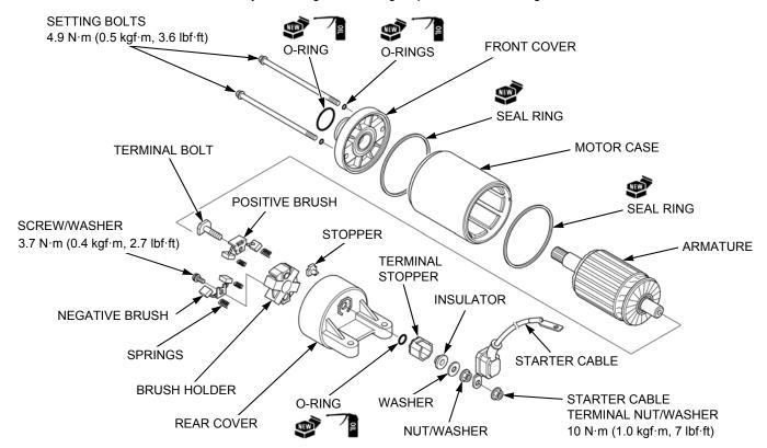
When installing the front cover [1] and rear cover [2] onto the motor case [3], align the lines as shown.
