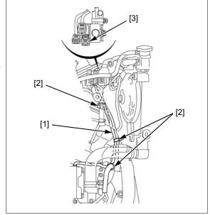
Remove the bolts [1] and linear solenoid valve body [2].
