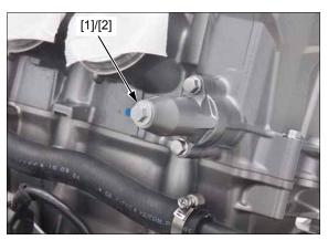
Turn the cam chain tensioner lifter shaft fully in (clockwise) and secure it using the special tool.
