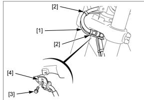
Remove the bolt [1] and front wheel speed sensor [2].
