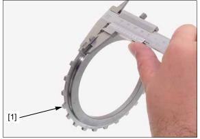
If the calculated dimension is over the thickest plate thickness, replace the clutch discs and plates as a set. Select the end plate from the table below.
