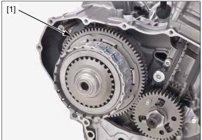
Remove the seal rings [1] from the mainshaft grooves.
