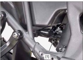
CRF1000: Release the turn signal light relay [1].
