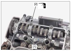
Remove the camshaft holders and measure the compressed plastigauge at its widest point on the camshaft to determine the oil clearance.
