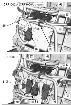
Install the connector cover [1] by aligning its bosses [2] and slit [3] with the connector clip stay holes and tab.
