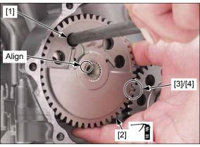
Install the special tool between the front balancer drive and driven gears.
