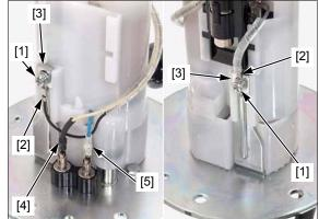
Remove the fuel pump filter assembly [1] and O-ring [2] from the fuel pump stay [3].
