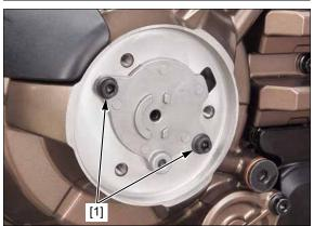
Install the inner clutch oil feed pipe [1] to the feed pipe guide plate by aligning the feed pipe bosses with the guide plate grooves.
