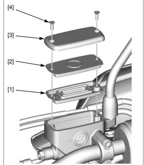
Rear brake: Remove the mounting bolt [1] and rear brake reserve
