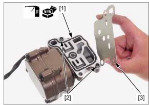
Coat a new packing [1] with engine oil and install it onto the spool valve filter [2].
