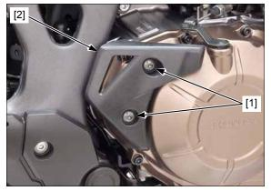
Loosen the lock nuts [1] and release the clutch cable [2] from the clutch lifter lever [3].
