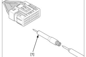
The ECM/PCM connector [1] terminals (wire harness side) are numbered as shown in the illustration.
