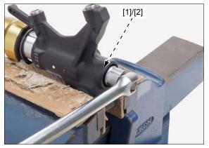
Remove the fork damper assembly [1] and centering plate [2].
