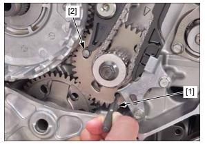
Remove the washer [1] and clutch outer [2].
