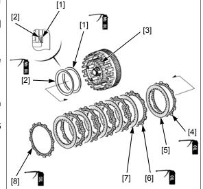
Install the clutch lifter pin [1].
