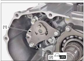
Install the drum shifter collar [1] onto the drum shifter.
