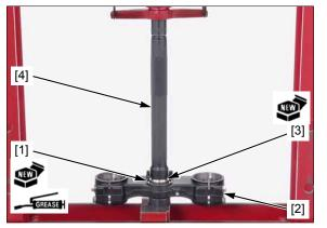
Drive in a new upper outer race [1] using the special tools.
