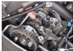
Adjust the No.2 cylinder exhaust valve clearance by loosening the lock nut [1] and turning the adjusting screw [2] until there is a slight drag on the feeler gauge [3].
