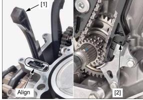
Install the dowel pins [1] and a new gasket [2].
