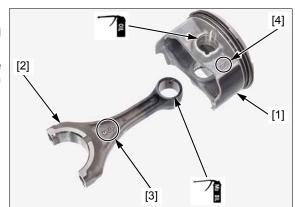
Apply molybdenum oil solution to the piston pin outer surface.
