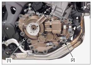
Coat a new O-ring [1] with engine oil and install it onto the water pipe [2].
