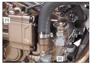
Connect the linear solenoid valve 4P (Black) connector
