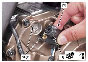
Install the bolt [1] and tighten it to the specified torque.
