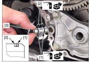
Install the dowel pins [1] and new gasket [2].
