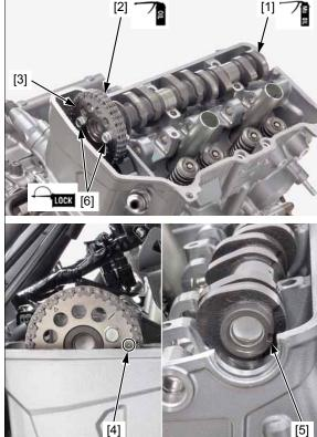
Apply molybdenum oil solution to the camshaft holders inside and install them in their original locations.
