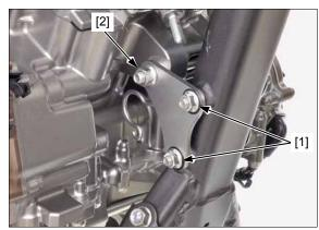
Tighten the front upper bolt (right side) [1] first, then the left side bolts [2] to the specified torque.
