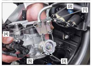
Disconnect the TP sensor 3P (Black) connector [1] and remove the throttle body [2].
