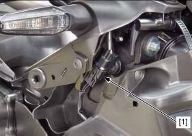
Remove the screw [1] and open air temperature sensor
