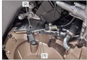
Install the bolts [1] and engine right side rear cover [2] and tighten the bolts to the specified torque.
