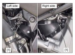
Disconnect the MAP sensor 3P (Black) connector [1]. Disconnect the IACV 4P (Black) connector [2].
