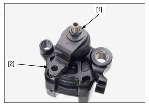
Apply 0.4 g minimum of silicone grease to the bracket and caliper pin boot insides.
