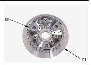
Check the following of the clutch outer [1] for scratch, damage, abnormal wear and deformation.
