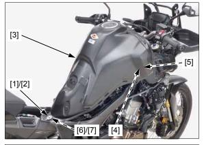
Check the fuel line [1] for deterioration, damage or leakage. Replace the fuel line if necessary.
