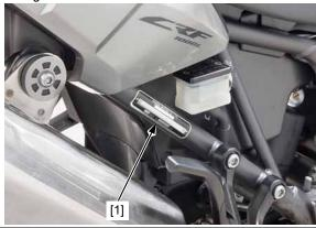
The compliance label (U model only) [1] is attached on the front side of the down tube.
