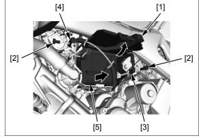
Connect the positive (+) terminal first and then the negative (-) terminal.
