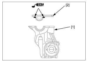
Check that the mounting rubbers [1] are in good condition, and replace them if necessary.
