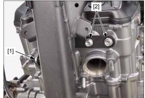
Tighten the rear upper bolts (8  $\times$  25 mm) [1] to the specified torque.
