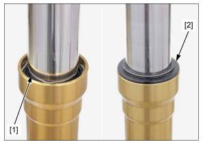
Install the fork damper assembly [1] and centering plate [2].
