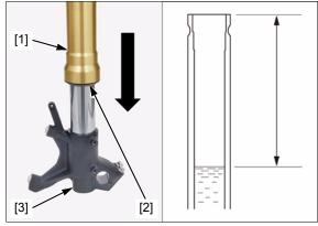
Install the fork spring [1] into the slide pipe assembly with the tightly wound side facing down.
