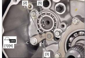
Hold the stopper arm [1] using a screwdriver.
