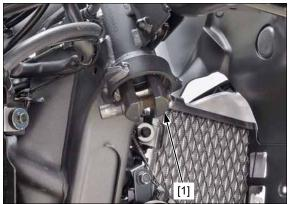
Temporarily install the steering stem nut [1] onto the steering stem [2] to prevent the threads from being damaged when removing the lower inner race [3] from the steering stem.
