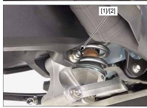
Remove the swingarm pivot nut [1], pivot bolt [2], and swingarm [3].
