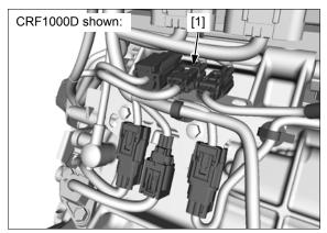
Remove the bolt [1] and sidestand switch [2]. Installation is in the reverse order of removal.
