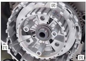
Line up the primary drive gear and sub gear teeth by inserting a suitable pin [1] into the holes of gears.
