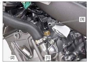
CRF1000/A: Remove the bolt [1] and clutch cable holder [2].
