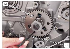
Temporarily install the clutch outer [1].
