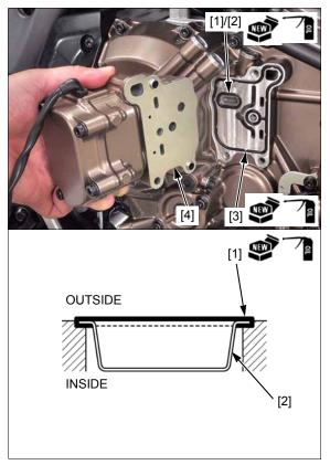
Install the bolts [1] and tighten it to the specified torque.
