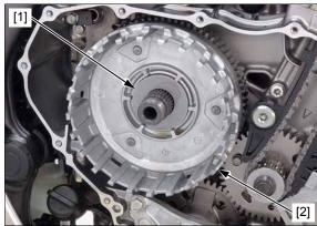
Remove the washer [1] and clutch outer guide [2].
