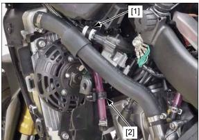
CRF1000D: Release the wire band [1] and clamp [2]. Release the clamp [3].
