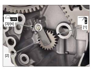
If you are replacing the rear balancer driven gear and/or needle bearing, record the corresponding balancer driven gear I.D. code [1] from the balancer weight.
