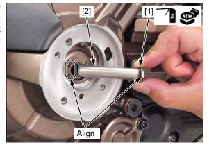
Apply engine oil to new O-rings [1] and install them to the feed pipe guide plate grooves.
