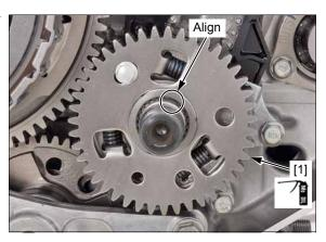
Apply engine oil to the primary drive gear nut threads and seating surface.
