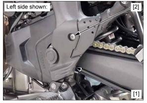
Install the drive chain case [1] and socket bolts [2] and tighten the bolt securely.
