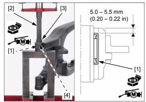
Apply molybdenum disulfide grease to a new needle bearing (24 x 31 x 28 mm) rotating area.
