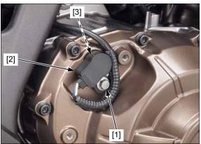
Remove the bolts [1] and clutch EOP sensor cover [2].
