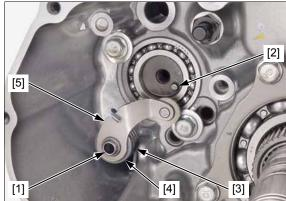
Hold the shift drum stopper arm [1] with a screwdriver and install the shift drum center [2] by aligning the groove [3] with the dowel pin [4].
