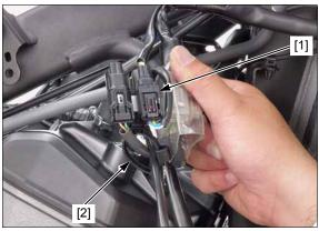
CRF1000D: Remove the bolts [1] and clutch EOP sensor cover [2].
