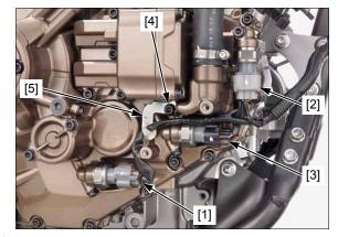
CRF1000D: Disconnect the EOT sensor 2P (Black) connector [1].
