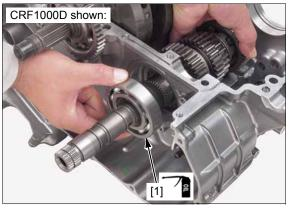
Apply locking agent to the mainshaft bearing set plate bolts threads (page 1-20).
