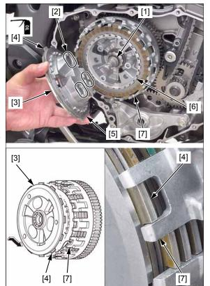
Install the clutch springs [1], set plate [2] and set plate bolts [3].
