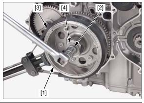
Remove the flywheel [1] using the special tool.
