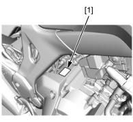
The throttle body identification number [1] is stamped on the upper front left side of the throttle body as shown.
