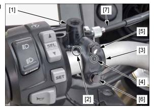
Connect the parking brake switch connectors [1]. Install the knuckle guard (page 2-5). Install the rearview mirror (page 17-10).
