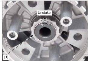
Install special tools and loosen the clutch center lock nut [1] while holding the clutch center with the special tool.
