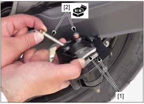
Install the parking brake caliper [1] and new mounting bolts [2] and tighten the bolts to the specified torque.
