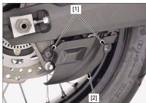
Remove the brake caliper mounting bolts [1] and caliper [2] from the bracket.
