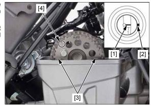
Check the No.1 cylinder intake valve clearances by inserting a feeler gauge [1] between the valve lifter and cam lobe.
