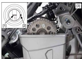
Check the No.1 cylinder exhaust valve clearances by inserting a feeler gauge [1] between the locker arm roller and cam lobe.
