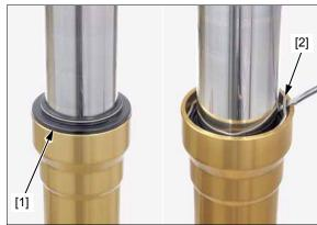
Pull the slide pipe assembly [1] out until you feel resistance from the slider bushing. Then move it in and out, tapping the bushing lightly until the outer pipe [2] separates from the slide pipe assembly.
