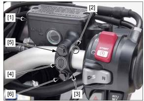
Install the wire clamp [1] and connect the front brake light switch connectors [2].
