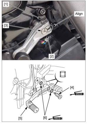
When adjusting the gearshift pedal height, perform procedures as follows:
