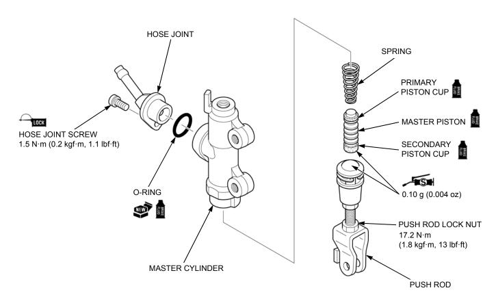
When the push rod has been disassembled, adjust the push rod length so that the distance from the center of the master cylinder lower mounting bolt hole to the center of the joint pin hole is standard length as shown.
