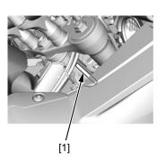
The engine serial number [1] is stamped on the lower back side of the crankcase.
