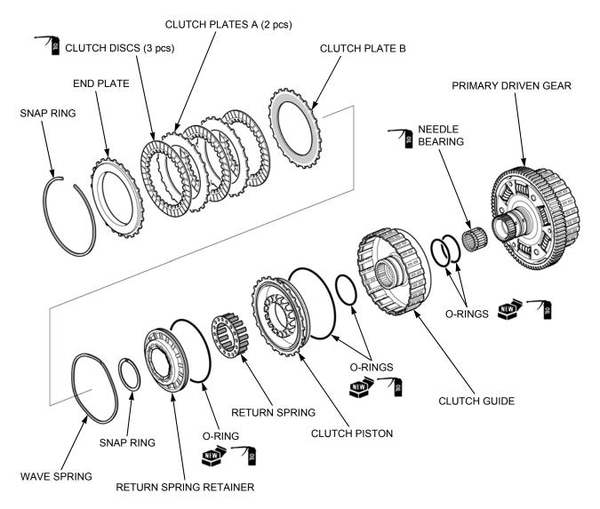
Clean the inner surface of the clutch guide thoroughly and blow through the oil holes.
