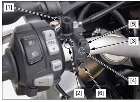
CRF1000D: Install the parking brake lever assembly [1] by aligning its end with the paint mark [2] on the handlebar.
