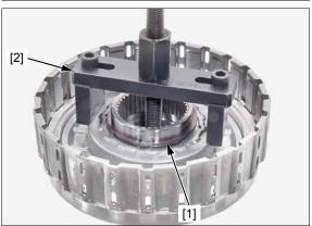
Remove the return spring retainer [1], O-ring [2], and return spring [3].
