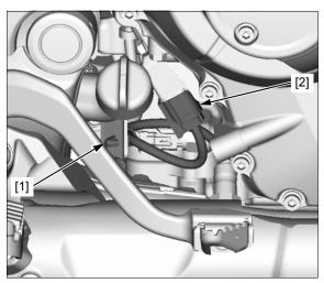
Remove the pan screw [1] and exhaust pipe cover A [2]. Loosen the band screw and remove the band [3] and exhaust pipe cover B [4].
