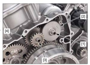
Hold the flywheel [1] using the special tool and loosen the flywheel mounting bolt [2].
