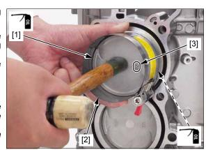
Make sure the piston ring compressor tool sits flush on the top surface of the
