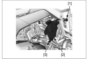
Release the starter relay switch [1] from the battery box. Remove the starter relay switch cover [2].
