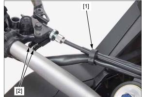
CRF1000/A: Remove the bolts [1], holder [2], and clutch lever assembly [3].
