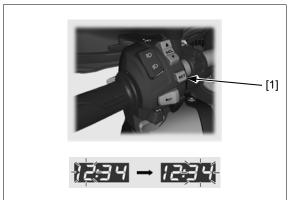
5. Press the UP [1] or DOWN [2] button until the desired minute is displayed.
