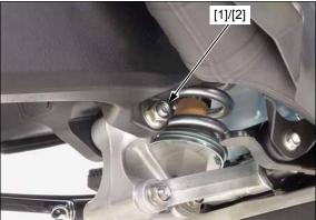
CRF1000D: Install the parking brake cable guide [1] and bolt [2].
