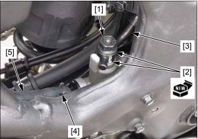
Remove the cotter pin [1] and joint pin [2], and disconnect the brake rod joint [3] from the middle arm
