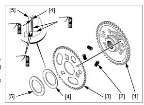
Place the snap ring [1] onto the front balancer driven gear assembly [2].
