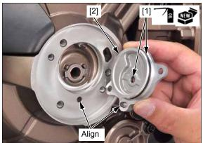
Install and tighten the bolts [1] to the specified torque.
