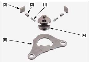
Install the drum shifter guide plate/drum shifter assembly [1].
