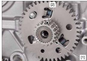
Temporarily install the clutch outer [1].
