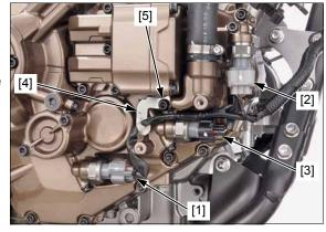
CRF1000D: Install the clutch EOP sensor cover [1] and bolts [2], and tighten the bolts to the specified torque.
