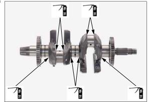
Be careful not to damage the crankpin, main journal and bearing inserts. Install the crankshaft [1] onto the upper crankcase and set the connecting rods onto the crankpins.
