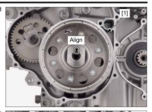
Apply engine oil to the flywheel mounting bolt threads and seating surface.
