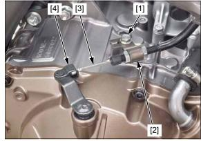
CRF1000D: Disconnect linear solenoid 4P (Black) connector [1]. Remove the wire band [2].
