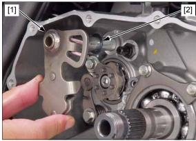
Remove the shift drum center bolt [1].
