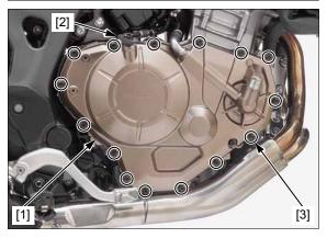
Connect the water hoses [1] and tighten the hose band screws [2] to the specified range (page 8-8).
