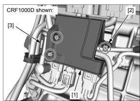
Disconnect the Alternator assembly 6P (Black) connector [1].
