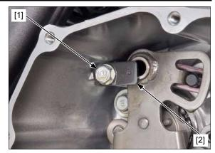
Pull the gearshift spindle assembly [1] and thrust washer [2] out of the crankcase.
