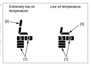
Turn the ignition switch ON with the engine stop switch "O" while pushing the D switch [1] of the N-D switch. The MIL [2] will come on.
