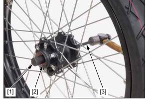
Never install the old bearings. Once the bearings have been removed, the bearings must be replaced with new Drive in a new left bearing [1] squarely with the marked side facing up until fully seated.
