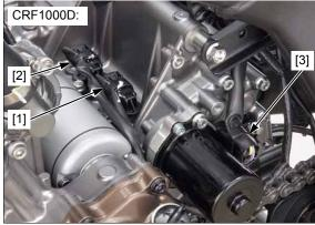
Loosen the hose band screw [1] and disconnect the radiator upper hose [2].
