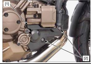
Apply engine oil to a new O-ring [1] and install it onto the shift spindle angle sensor [2].
