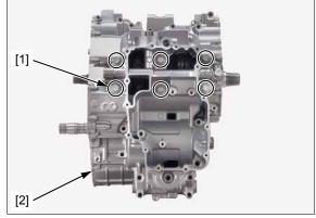
Remove the dowel pins [1], oil joint A [2], and oil joint B
