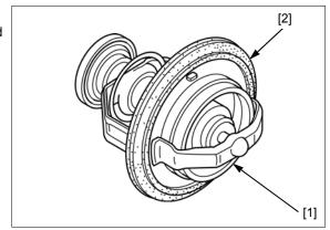
Visually inspect the thermostat [1] for damage. Replace the thermostat if the valve stays open at room temperature.
