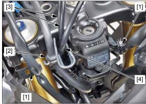
Remove the steering stem nut [1]. Remove the forks (page 17-14).
