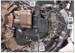
CRF1000D: Connect linear solenoid 4P (Black) connector [1]. Install the wire band [2].
