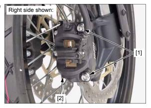
Remove the brake pads [1].
