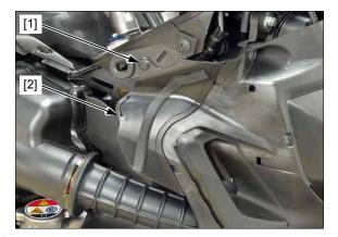
Disconnect the open air temperature sensor 2P (Black) connector [1].
