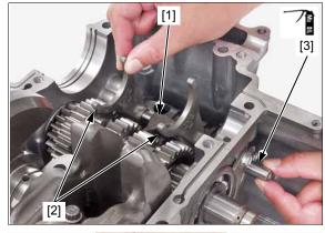
CRF1000D: Install the following with the identification marks facing toward the right side of the engine:
