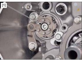
Remove the shift drum center [1] while holding the stopper arm [2] using a screwdriver as shown.
